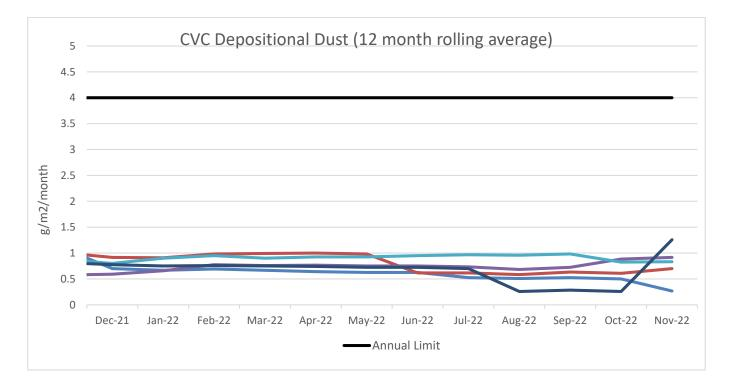
A 12-month rolling average of depositional dust concentrations has been presented below. Dust Gauges DDG001, DDG002, DDG003 and DDG004 are located within a closer proximity to Chain Valley Colliery and DDG006 is positioned in a location representative of the Chain Valley Colliery ventilation fan site at Summerland Point.
